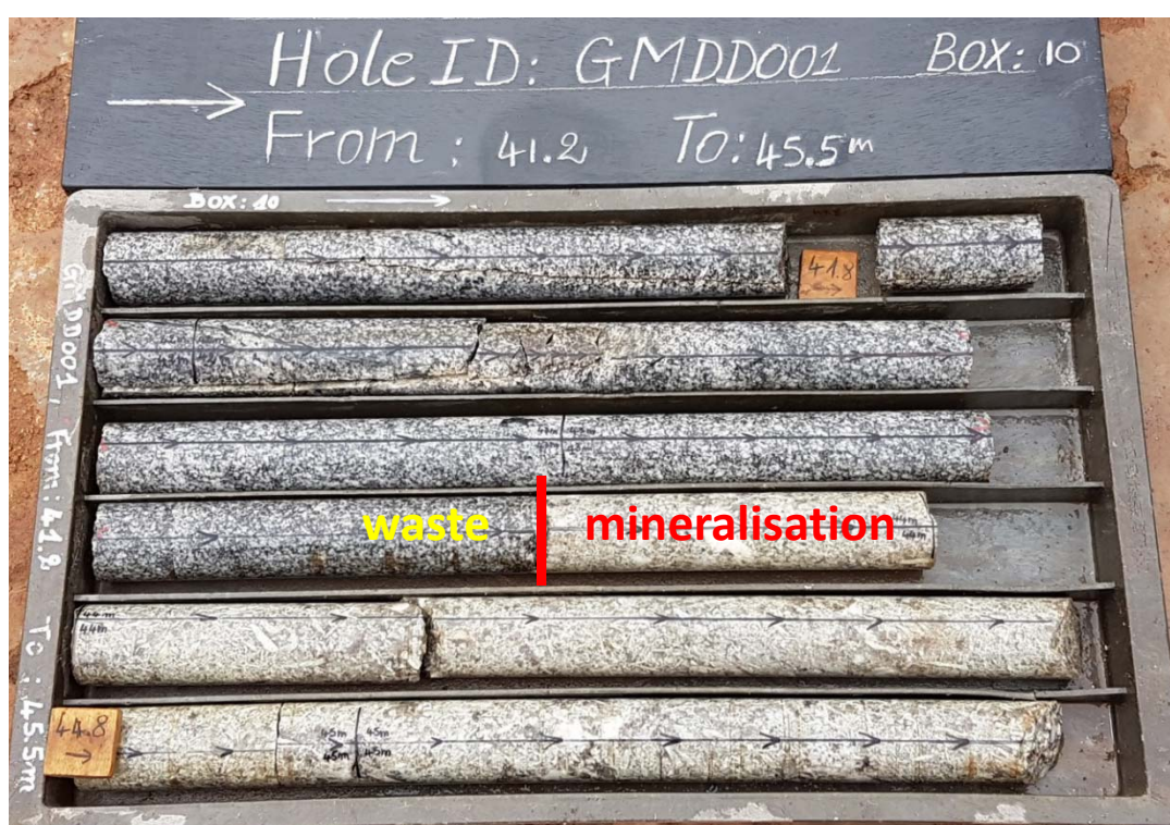
Figure 1. Image from drill core at Goulamina, showing sharp and visually distinct contact between biotite granite waste rock (dark) and mineralised pegmatite (white)
